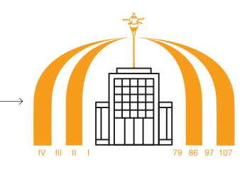
The level of protection is given using NFC 17-102 ed. 2011, or EN 62305-2, or using the FDC 17-108  $\,$ guide. If the site presents a risk for the environment the protection radius must be reduced of 40%. For a level of protection I++ [cf. 5.2.3.5 NFC 17-102], the radius of protection must be reduced of 40%.
