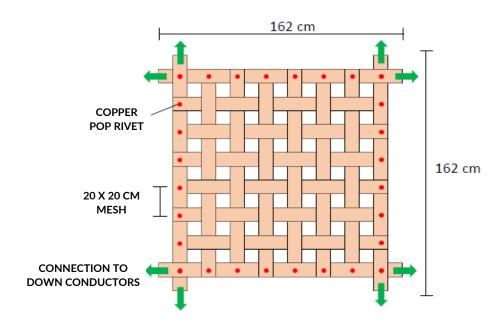
Example of the use of 4 earthing grids with flat/flat connection to the down conductor:
