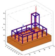
Some Perfect Match Layers (PML) [2] have been implemented around the calculation volume, and are like if the case studied was located in an infinite space. Indeed, the PML avoid reflections, and side effect of the calculation volume.
