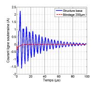
The lightning current applied only modelize the first strike. The mathematic formula used is one of a bi-exponential waveform with time parameters of 10/350µs, and a peak current of 200kA.
